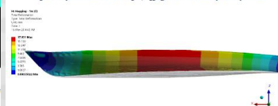
Figure 9. Deformation at 1m wave height (Sagging) with a maximum deflection of 25.2mm
